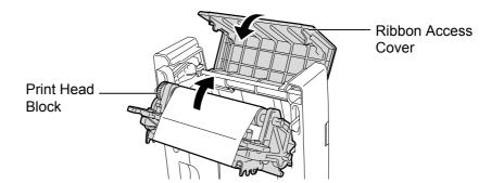
**7.** Again, turn the Ribbon Rewind Gear to remove any slack of the ribbon.
